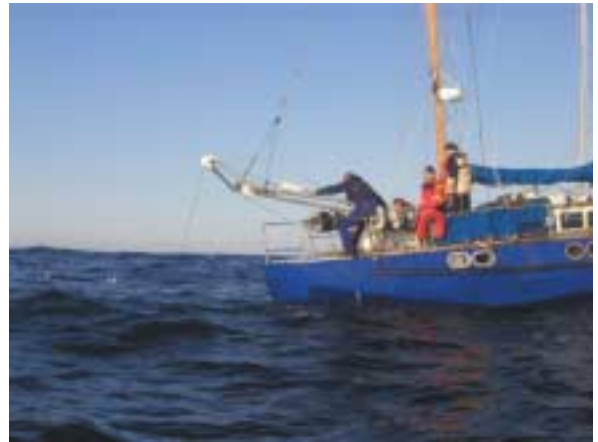
Fig. 6. The second pulley has lifted the canister over the first pulley. The canister now has to pass the winch. Photographer: S.F. Hansen.
