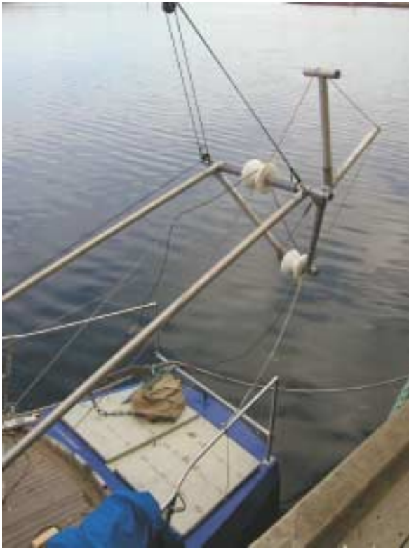
Fig. 4. The crane. The two pulleys can be seen and part of the suspension from the mast. Photographer: S.F. Hansen.
