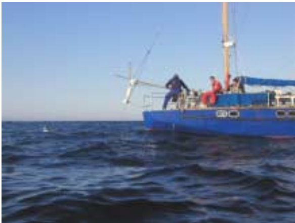
Fig. 5. A canister on its way up has reached the first pulley. The second pulley on the extension of the crane is being engaged. Photographer: S.F. Hansen.
