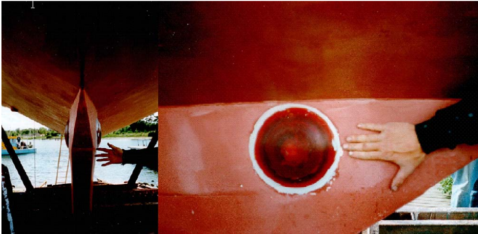
Fig. 2. Hydrophones mounted on r/v Narhvalen. Frontal and side view.
